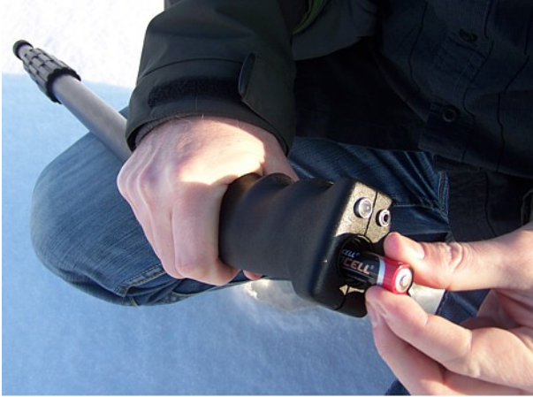
Figure 5.1: Insert the batteries into the telescopic antenna
