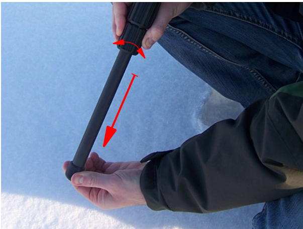
Figure 5.2: Extend the telescopic antenna
