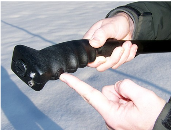
Figure 5.3: Turning on the telescopic antenna
