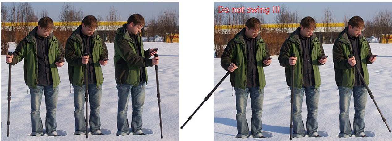
Figure 6.13: Discrimination with the telescopic antenna
