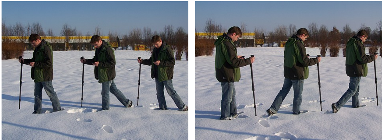
Figure 6.6: "Zig-Zag" scan in operating mode "3D Ground Scan"
