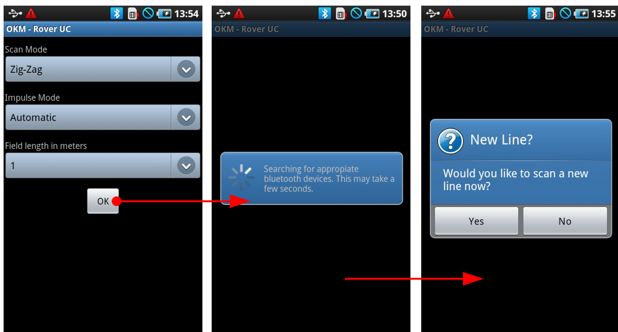
Figure 6.5: Establishing a Bluetooth connection in operating mode "3D Ground Scan"
